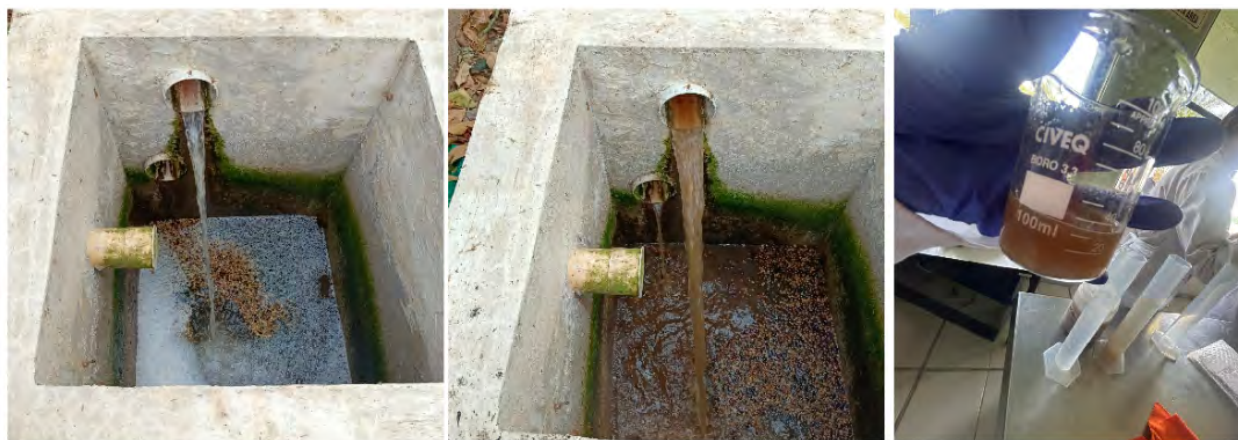
Figure 3. Discharge of community's municipal wastewater and coffee-processing wastewater
