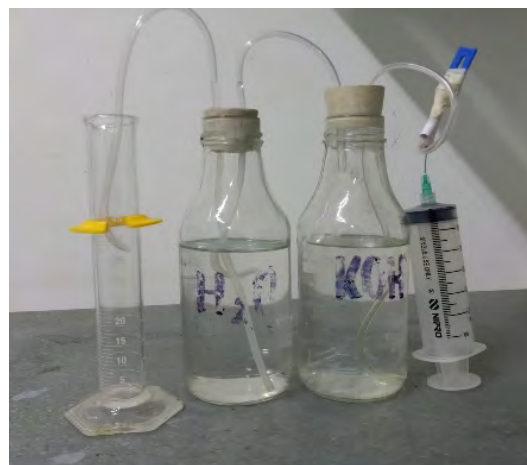
Figure 2. Mechanism of \text{CO}_2 removal from biogas
