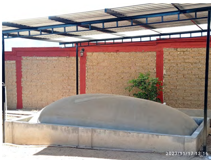
Figure 1. A tubular or bag-type biodigester with a liquid volume of 10 m 3 was used in the present study
