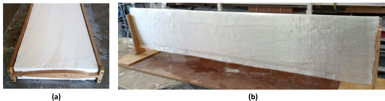
Figure 5. (a) Wood guides for EPS core, and (b) Biaxial fiberglass on EPS core.
