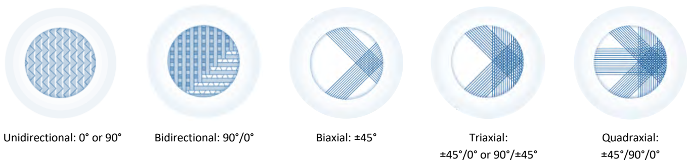
Figure 2. Typical orientation of continuous fiber reinforcements (Gurit, 2016).
