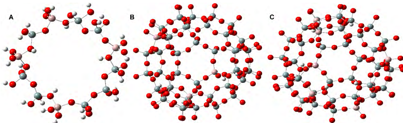
Figure 6. Models of HZSM5-type zeolites: A) Zeolite ring with four tetrahedral centers (4T); B) HZSM5 zeolite structure with a 50% ratio; C) HZSM5 zeolite structure with a 100% ratio. The O atom is colored red, the Si atom is gray, the Al atom is pink, and the H atom is white.
