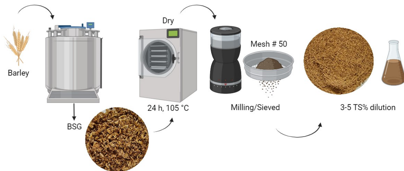
Figure 1. Proposed methodology for conditioning brewing waste obtained from the fermentation of craft beer.
