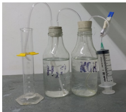
Figure 2. Mechanism of \text{CO}_2 removal from biogas
