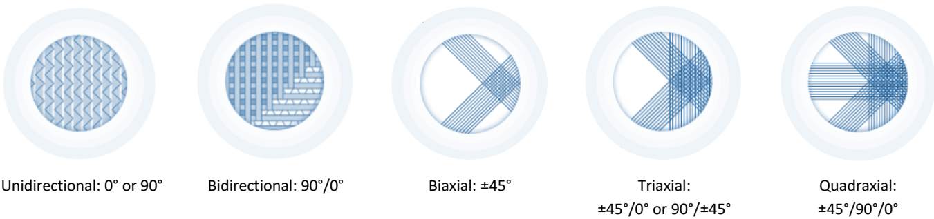
Figure 2. Typical orientation of continuous fiber reinforcements (Gurit, 2016).
