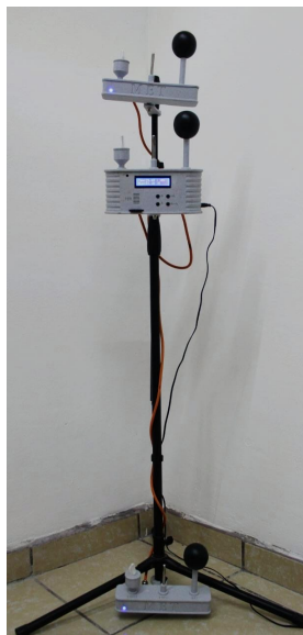
Figure 3. Electronic meter for high or low temperatures and relative humidity. (prototype)
